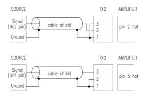
Figure 2. Input connections from an unbalanced source
